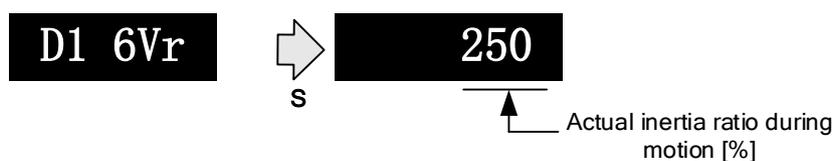
Use auxiliary function **AF\_GL** or Motion studio to measure the inertia ratio. The result will be shown on **D1 6Vr**, hold M to write the value in Pr0.04.
