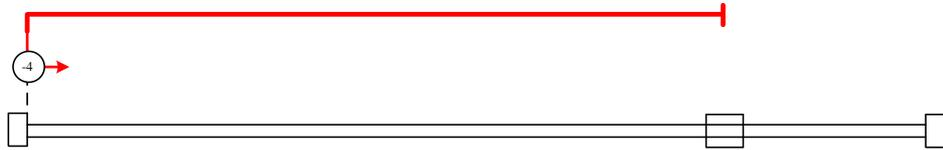
**Mode -3:** Search for homing point in **positive direction** at **high velocity**. Move in **negative direction** after torque reaches the value set in Pr5.39, stops when torque is gone. Homing done signal delivers after the time value set in Pr5.37
